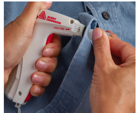
Pull trigger to attach fastener
