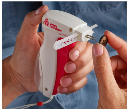
Load button onto needles
